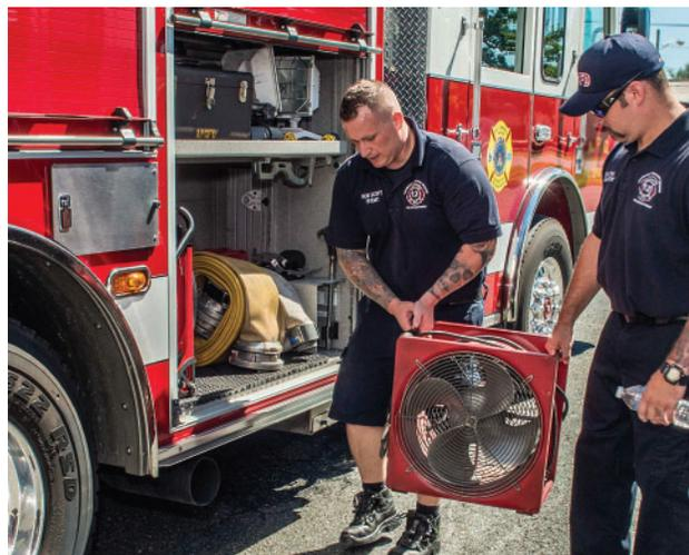
**Figure 15-11.** Firefighters relocate a smoke ejector fan after an ergonomic intervention. Notice how relocating the fan from the top of the fire truck to the rear bumper allows for easier access. Photograph courtesy of Christina Graber, Army Public Health Center, Aberdeen Proving Ground, MD. Used with permission.
