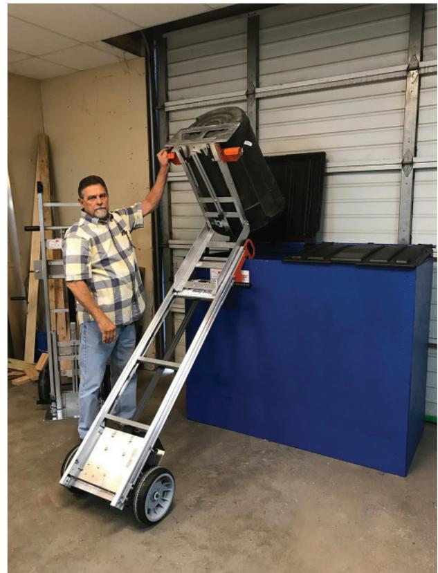
**Figure 15-9.** Waste removal process after an ergonomic intervention. Notice how the use of an engineering control reduces the risk of worker injury.
